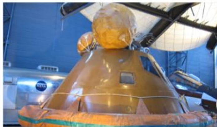
The Columbia Command Module has a custom made flotation collar to help it float when it landed in the Pacific Ocean.
